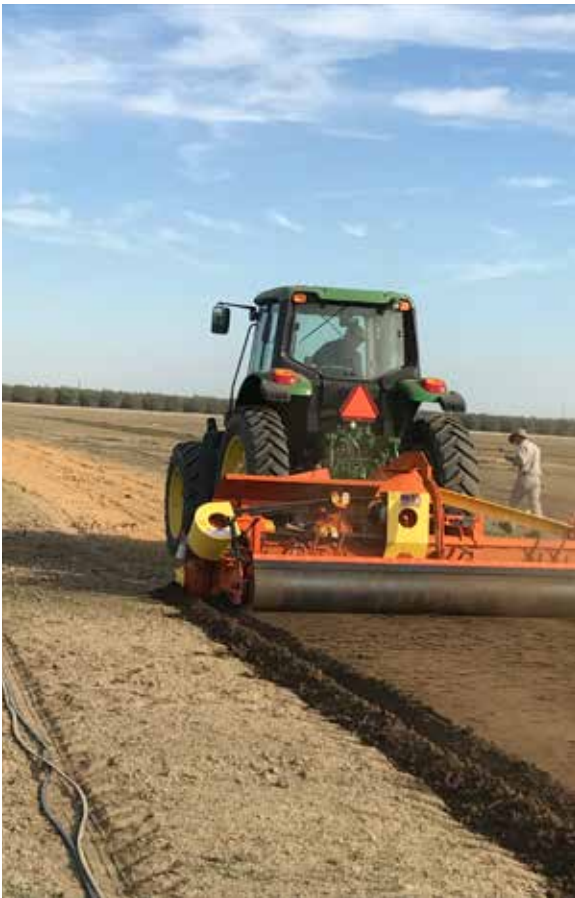
Figure 4. Incorporation of wood chips and ASD substrate (ground almond hull and shell) into the soil using a Northwest Tiller rototiller.
