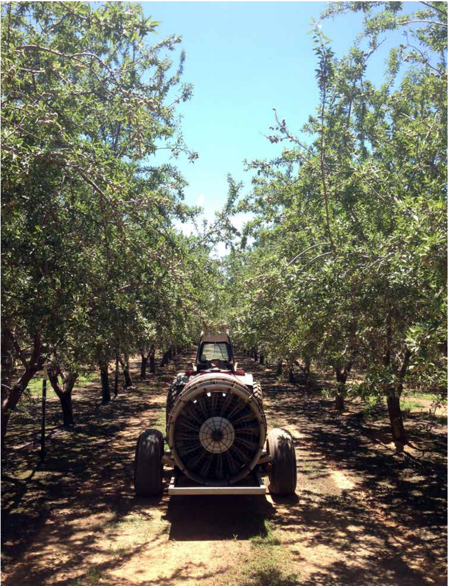
A key step to directing spray is to just park the sprayer in the orchard and look at what nozzle sites are pointing at what part of the tree.
