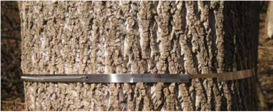
Dendrometer band on tulip poplar tree, photo courtesy Smithsonian Environmental Research Center's Global Tree Growth Project.
