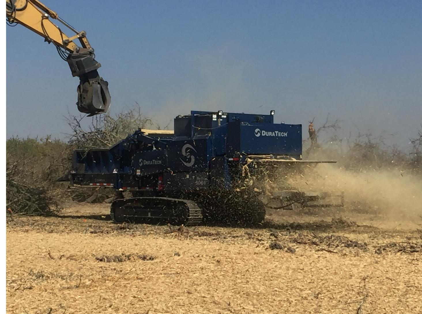
This Duratech grinder is mobile and spreads the wood chips evenly as it grinds.
